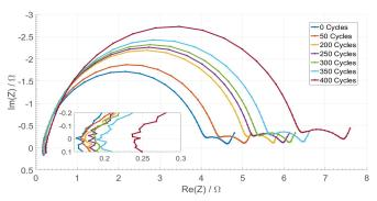
Spectrum of cell manufactured at Battery LabFactory clearly shows
